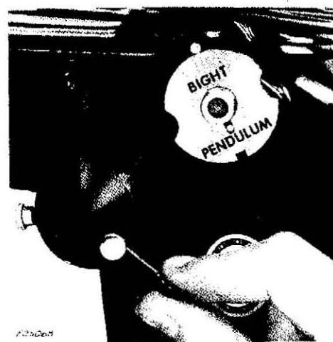
Fig. 98. Vibration Gauge Test While Swinging Lever to Full Bight
