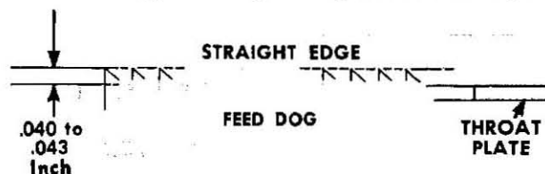
Fig. 274. Feed Dog at Correct Height
