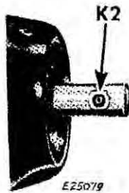
Fig. 32. Screw Seat Near End of Arm Shaft
